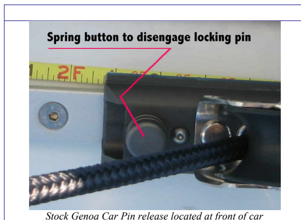
Stock Genoa Car Pin release located at front of car
