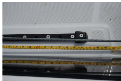
Car location when reefed to the second mark 32" forward
