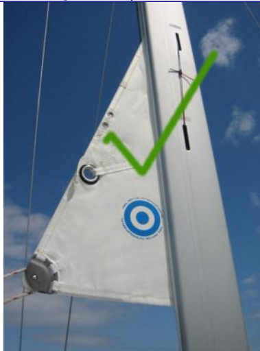
Mainsail with label furled inside mast and sail furled correctly.
