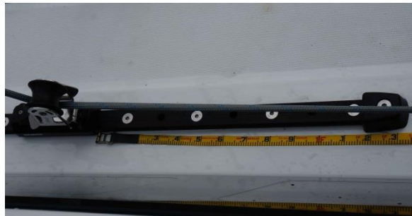
Car location when reefed to the first mark 16" forward.
