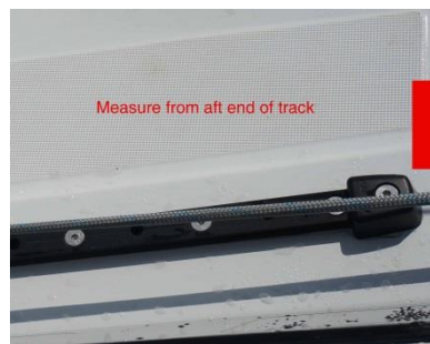
Measure from aft end of track forward to aft end of car
