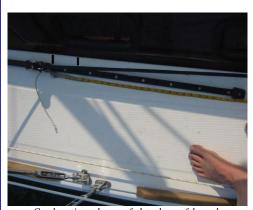
Car location when reefed to the reef 1 mark. Note both marks on the deck for full size and reef 1
